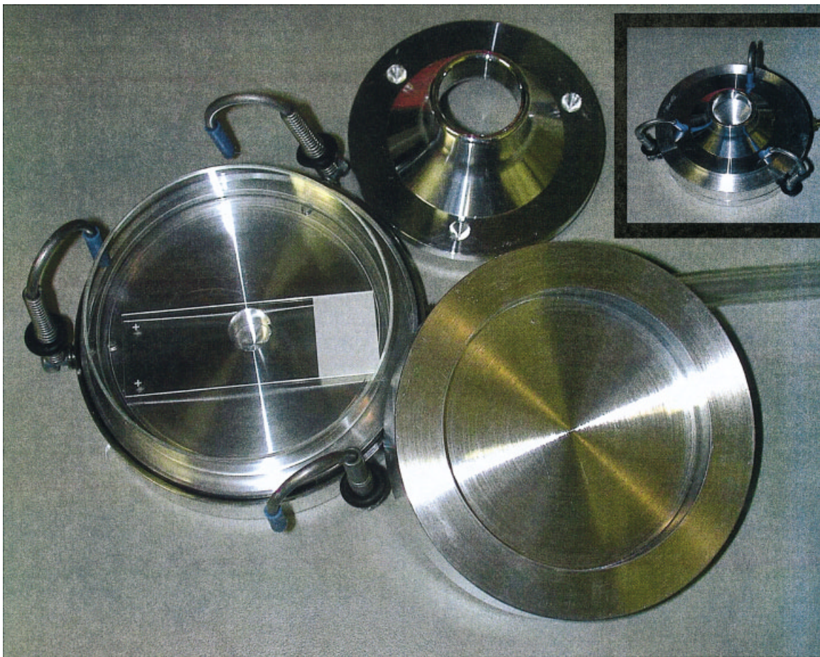
FIG. 3. AeroTech collection device. This picture shows the device in separate parts and assembled (inset). The AeroTech collection system consists of the base plate, the middle holed plate, and a funnel plate. The base plate holds a Petri dish, where a glass slide can be placed to detect the Glo-Germ particles. The middle plate is placed on top of the base and contains 400 precision holes, which produce a characteristic pattern if large amounts of aerosols are present. The top plate contains a funnel, where aerosols are forced down through the holes and onto the glass slide.
